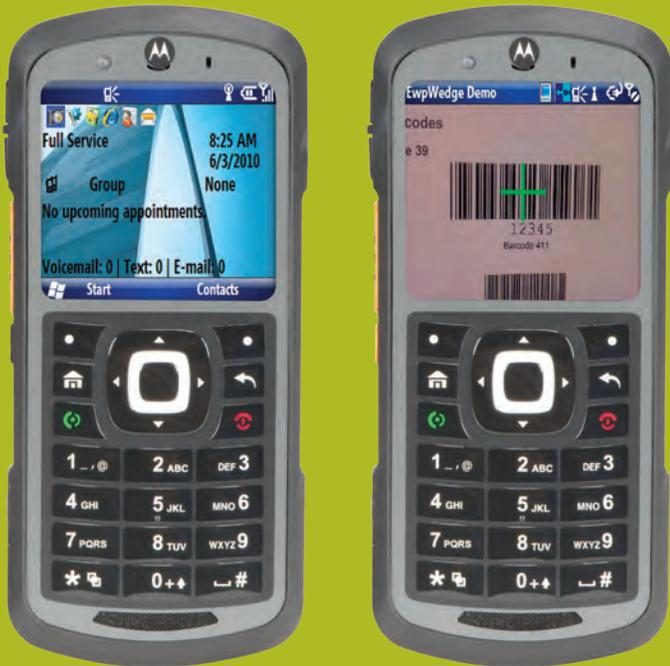
Give your workers a single pocketable device for all communication needs inside the Enterprise with Motorola's TEAM VoWLAN smartphones. The EWP2100 semi-rugged VoWLAN smartphone is built to endure the demands of everyday use in the enterprise, offering sealing against moisture and dust, a rigorous 4 ft./1.2 m drop specification that meets military standards (MIL-STD 810F) and a keypad that can be wiped clean.
